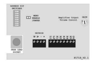
Network Terminals: Connect to the Intercall 700 4 wire Network. [A,B,+,-] OBSERVE POLARITY
