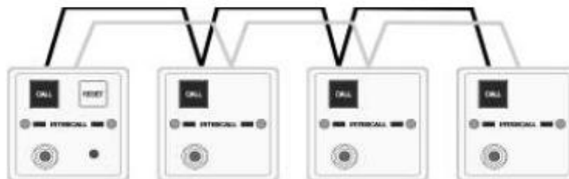
Max 3 SCP may be used to trigger a single call point
