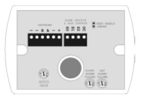
Network Terminals: Connect to the Intercall 700 (4 wire) Network. [+, -,A,B] Additional terminals are provided
