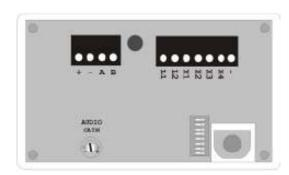
Network Terminals: Connect to the Intercall 700 four wire Network. [A,B,+, -] OBSERVE POLARITY
