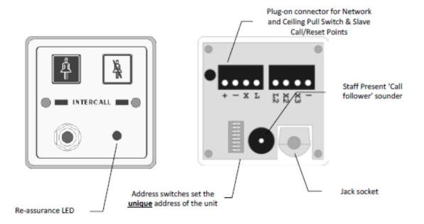
Network Terminals: Connect to the Intercall 600 (2 wire) Network. [+, -] OBSERVE POLARITY
